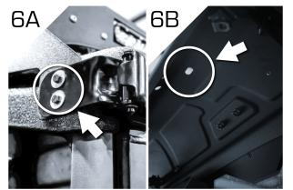
**NOTE:** Rear of roof will be marked with white dots to drill through. RTV Silicone is recommended to be applied under washers before securing back to roof to prevent any future leaks.
